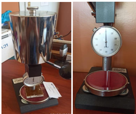
Fig. 2. Shore-D test device.
