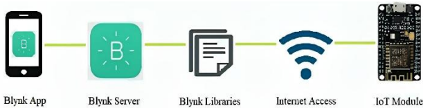
Fig. 2. Blynk working principle
