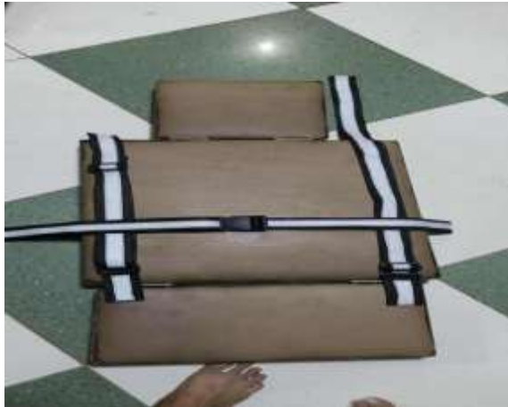
Fig. 3. Fully assembled padded deck, headrest, and adjustable restraint harness system of the mechanics creeper.
