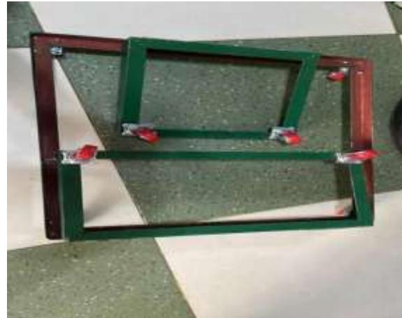
Fig. 4. Bottom view showing the structural frame layout and caster wheel placement of the improvised mechanics creeper.
