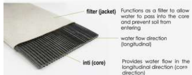
Fig. 4. Prefabricated Vertical Drain [29]
