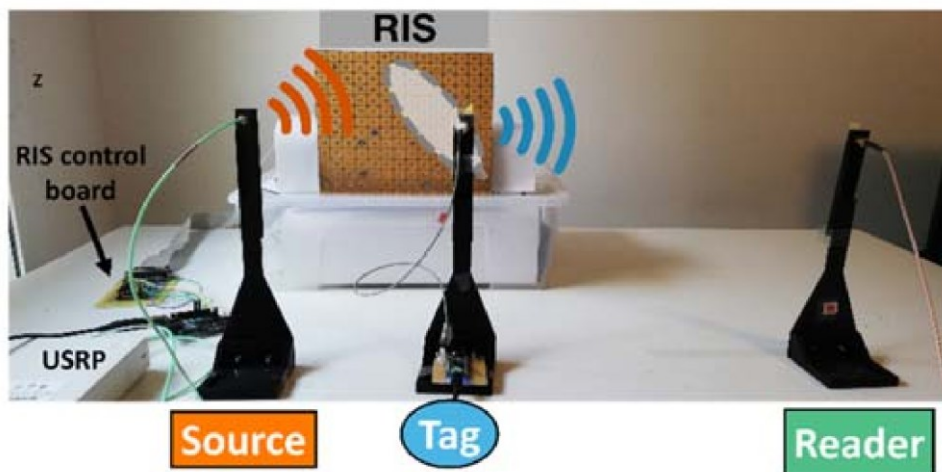
Fig. 5. Illustration of the considered testbed for RIS-assisted AmBC in [9].
