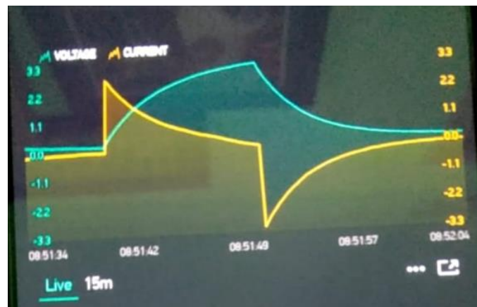
Fig. 8. Resulted visualization of transient phenomena of capacitor on smartphone, voltage (green) and current (yellow).
